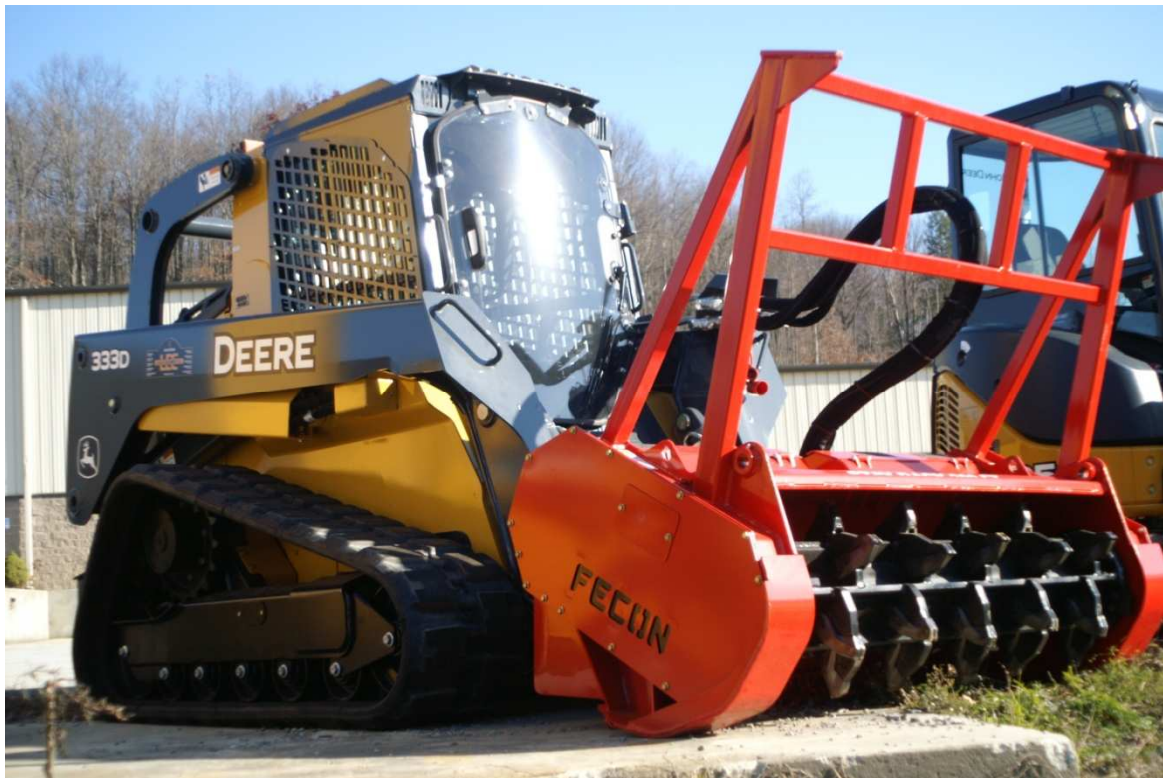
Figure 2. Specially equipped skid-steer loader with brush mulching attachment for treatment of large woody non-native invasive species
